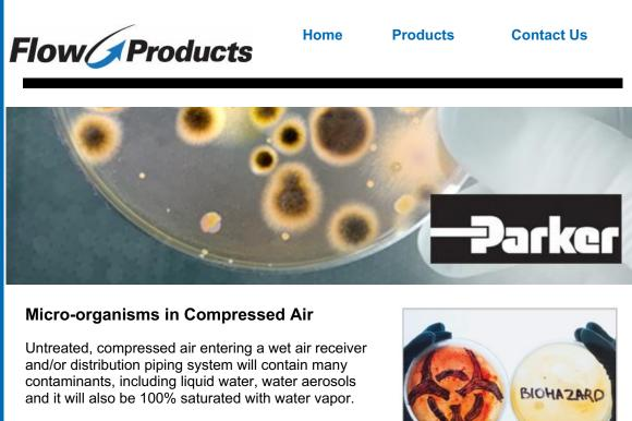
Water is the most problematic of all compressed air contaminants as it not only causes damage through corrosion, more seriously; wet compressed air promotes the growth of micro-organisms.
